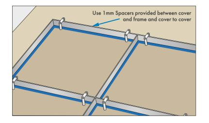
6 Next, the covers should be placed into position, the cover securing bolts should be screwed in (finger tight only) and the 1mm spacers provided should be inserted between the cover and frame at regular intervals to maintain a nominal 1mm gap between the covers and outer frame.
